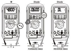
Normal forward voltage drop (forward biased) for a good silicon diode is between 0.400V to 0.900V. A reading higher than that indicates a leaky diode (defective). A zero reading indicates a shorted diode (defective). An OL indicates an open diode (defective). Reverse the test leads connections (reverse biased) across the diode. The digital display shows OL if the diode is good. Any other readings indicate the diode is resistive or shorted (defective).
