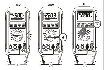
Note: Input sensitivity varies automatically with function range selected before activating the Hz function. mV function has the highest (300mV) and the 1000V range has the lowest (300V). It is recommended to first measure the signal voltage (or current) level
